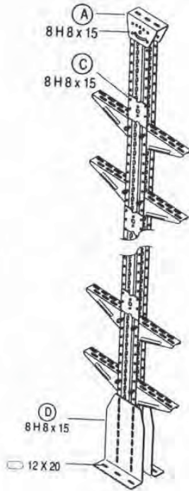
Double hanging system with one-way brace.
